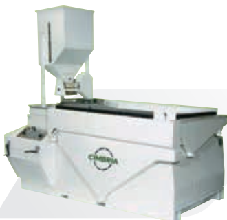
GA 210 Deck surface of 3,4 m 2
