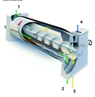
Through the inlet housing, the granular material to be graded flows into the interior of the rotating cylinder whose cover is provided with special deep drawn "tear-drop or spherical" shaped pockets for the most precise length separation.
