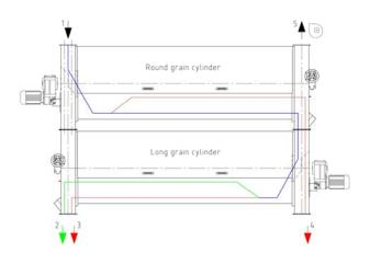
The grains that embed themselves fully into the indents, will be lifted and after a certain distance (adjustable to suit) will fall out of the pockets under gravity into the trough (Trough-Product) and will be discharged by means of a conveying screw.
